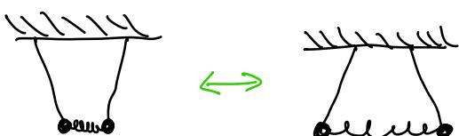
Mode 2: Spring compresses and expands, higher frequency of oscillation.
