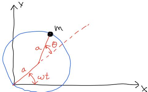
$$\text{Center of hoop: } x_c = a \cos(\omega t) \quad y_c = a \sin(\omega t)$$
