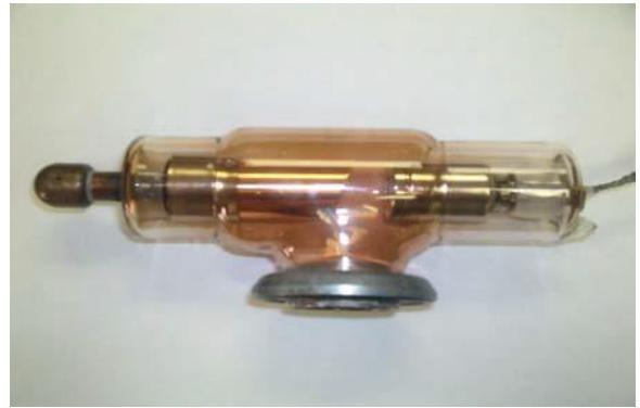
The spinning anode tube design is used in many diagnostic X-ray systems. The anode spins or rotates at high speed during X-ray exposure. This design permits the produced heat to be distributed over a much larger area, allowing a corresponding increase in X-ray production and reduction in exposure times.
