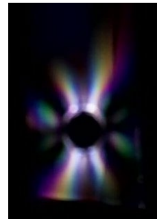
Figure 4 – Photoelastic effect of MTS \frac{1}{4} " plexiglass test
