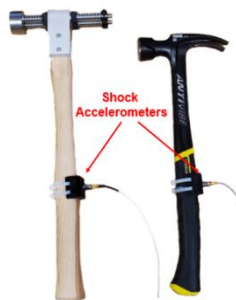
Figure 3: Testing Setup of Hammers
