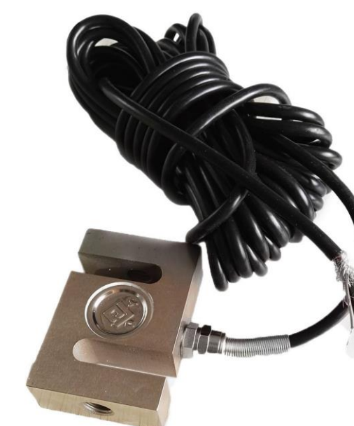
Figure 5: 500kg s-beam load cell used to record actuator load
