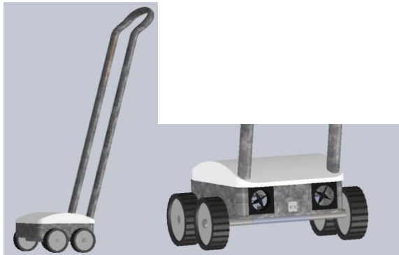
Figure 2. Design of R0V3R with casing and conduit handle
