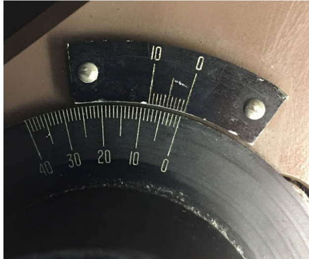
Figure 9: Adjustable Polarizer Dial
