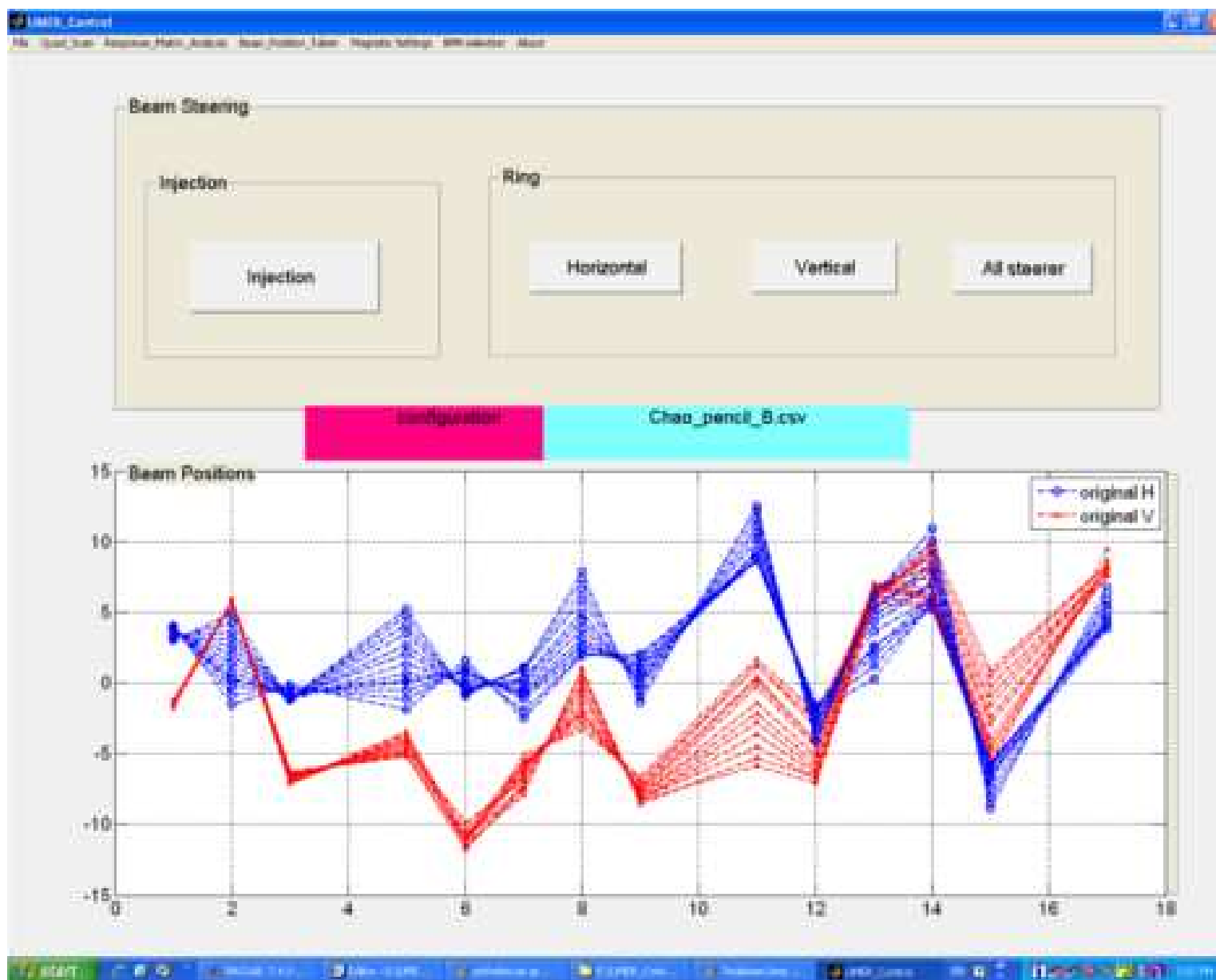
Figure 2.10: This is a screenshot of the GUI for the automated beam position monitor recording program. The blue line shows the horizontal and the red line the vertical excursion from the centerline of the BPM.
